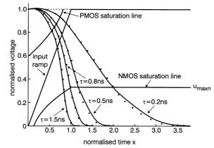
Fig.5 Inverter output waveforms for several values of input rise time analytical
