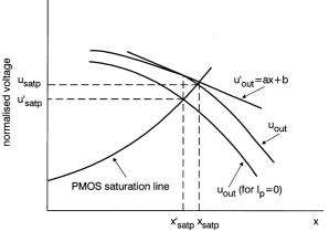
Fig.3 Evaluation of normalised time  $x_{satp}$  where inverter is entering region 3
