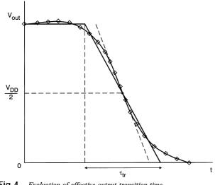
*Evaluation of effective output transition time* ramp approximation of  $V_{out}$ Fig.4  $\diamond$ V<sub>out</sub>
