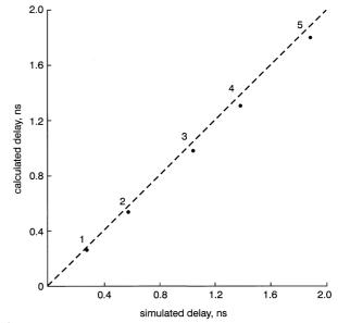
Fig.8 Comparison of calculated and simulated chain delay
