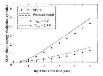
Fig. 12. Inverter short-circuit energy dissipation during one switching cycle, for two values of supply voltage ( $V_{\rm DD} = 2.5$  V,  $V_{\rm DD} = 5$  V).
