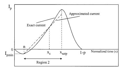
Fig. 3. Linear approximation of the PMOS current in region 2.
