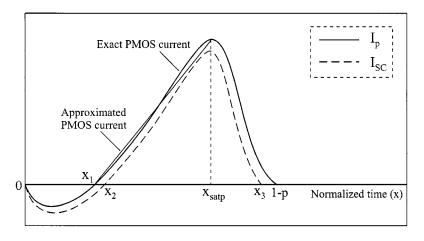
Fig. 4. PMOS and short-circuit current waveforms of the inverter.
