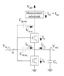
Fig. 15. Measurement of short-circuit energy dissipation in CMOS structures for a falling output waveform.
