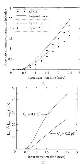
Fig. 11. Inverter short-circuit energy dissipation (a) and contribution of the short-circuit energy to the total energy dissipation (b) during one switching cycle, for two values of output load ( $C_L = 0.2$  pF,  $C_L = 0.1$  pF).
