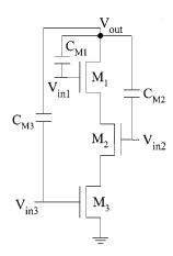
Fig. 9. Contribution of series-connected transistors (when they operate as short-circuiting block) to the gate equivalent input-to-output coupling capacitance.
