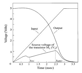
Fig. 7. Voltage waveforms of a three-input NAND gate for slow inputs.
