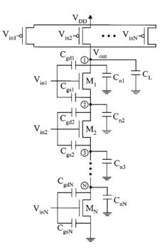
Fig. 5. Multiple-input static CMOS gate.
