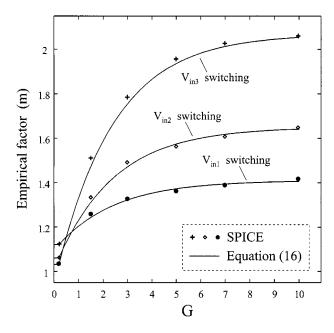
Fig. 8. Empirical factor m as a function of  $G = (I_{\text{DON}}\tau)/(V_{\text{DD}}C_L)$  for a three-input NAND gate.
