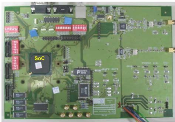
Fig. 7. Reference board hosting the implemented SoC
