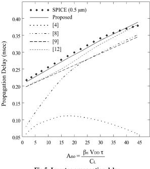
Fig.5: Inverter propagation delay
