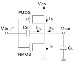
Fig.1: The CMOS inverter
