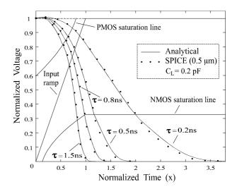
Fig.4: Inverter output waveforms
