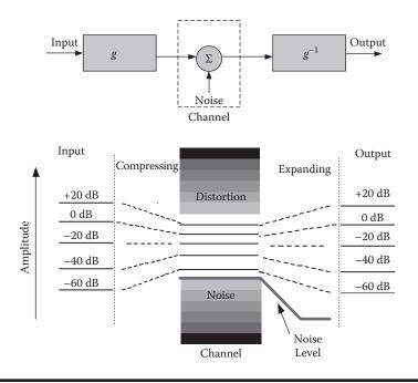
Figure 10.5 The instantaneous companding principle.
