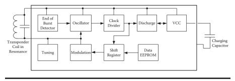
Figure 10.2 Typical block diagram of an RFID tag.
