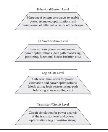
Figure 10.7 Power-oriented design flow with power analysis and optimization steps.
