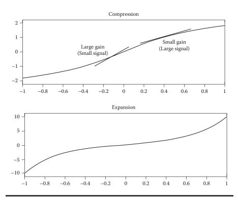
Figure 10.6 Appropriate, signal-dependent shapes for instantaneous companding.
