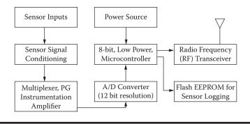
Figure 10.1 A block diagram of a typical wireless microsensor node.
