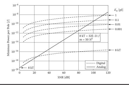
Figure 10.4 Minimum power consumption of analog and digital circuits.
